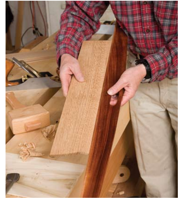
Here I'm using my shop-made straightedge to check the edge of the tongue for true.
