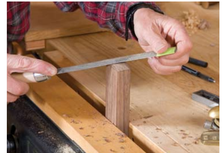
I smooth the radius with a series of rasps and files.
