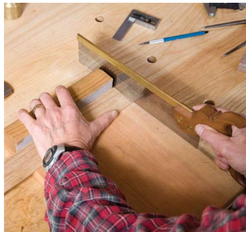
With the tongue held in a bench hook set on my joinery bench, I cut the tongue to precise length with a crosscut backsaw.
