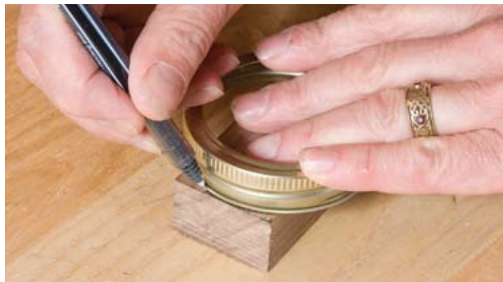
For a decorative touch, I often curve the bottom of the handle, laying it out to a radius similar to the radius at the end of the tongue. Here a jar lid is close enough!
