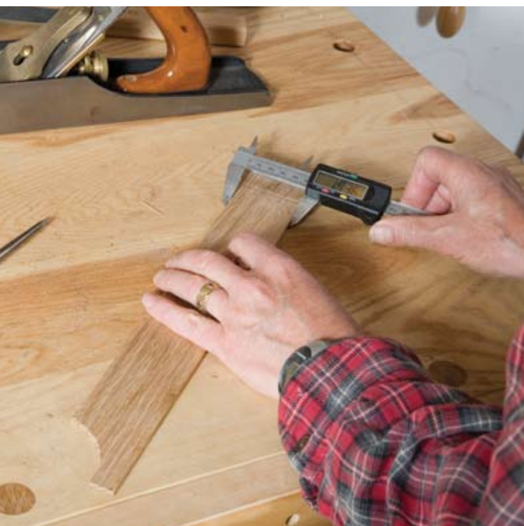
To ensure that the two edges of the tongue are precisely parallel, I measure their width with a caliper at each end of the board. I'll trim one edge as necessary until I get them parallel within a couple thousandths of an inch.
