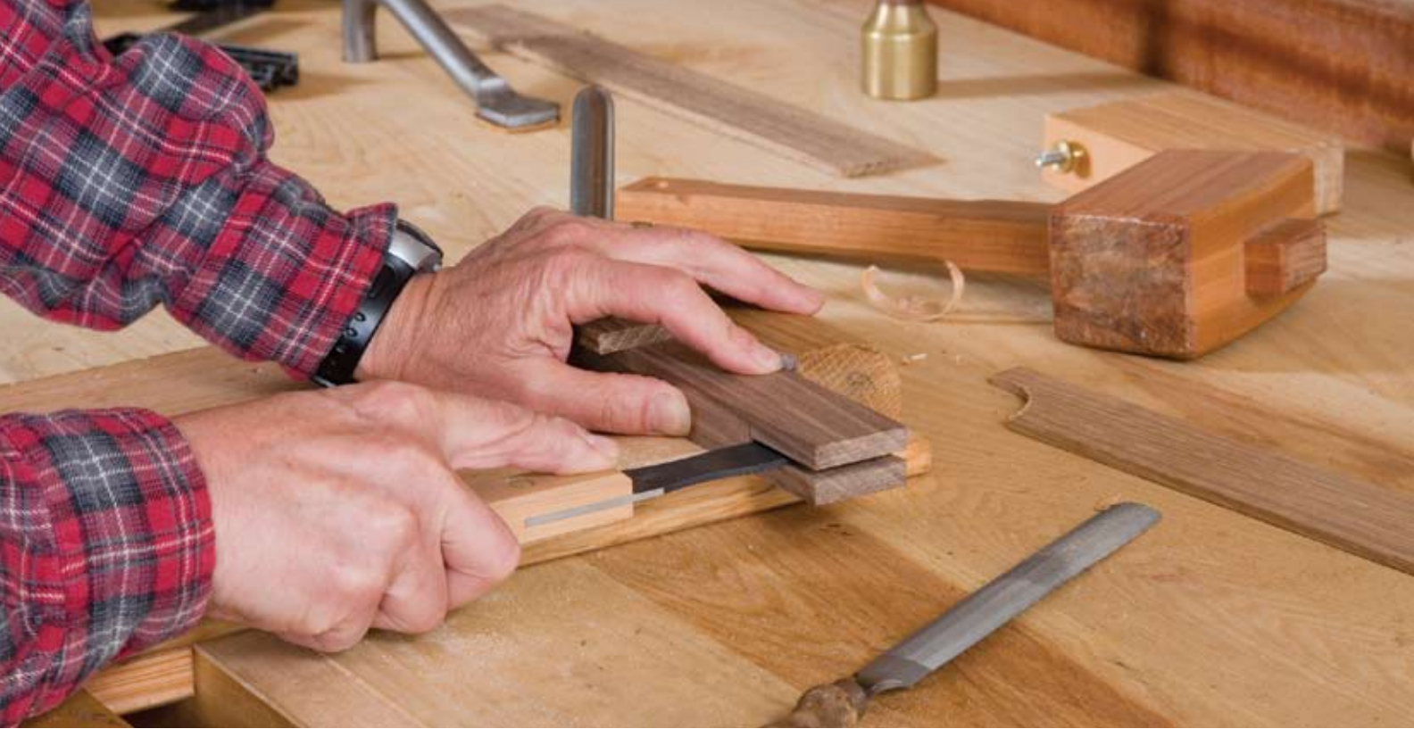
To pare the sides of the bridle joint to fit the tongue stock, I use a float or a cabinetmaker's rasp, testing the fit after every few strokes.
