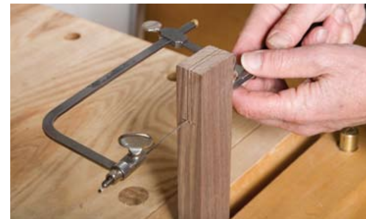
CUTTING OUT WASTE WITH A COPING SAW — THREE STEP PROCESS
