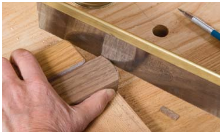
For a decorative touch, I often curve the bottom of the handle, laying it out to a radius similar to the radius at the end of the tongue. Here a jar lid is close enough!
