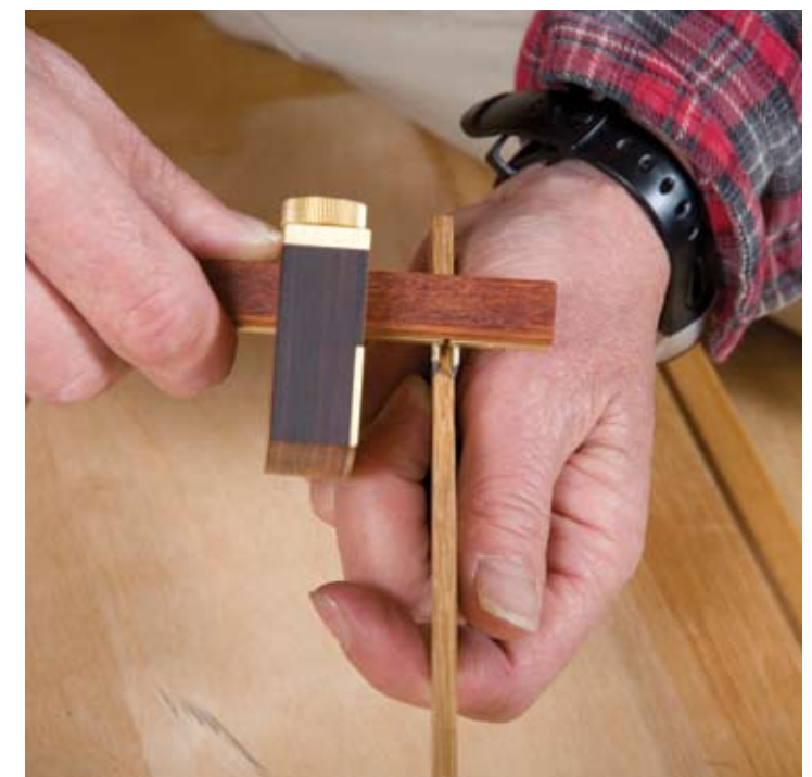
To layout the bridle joint that will accept the tongue, I set the dual pins of a mortise gauge to the width of my 1/4" chisel — which is slightly narrower than the thickness of the tongue stock.
