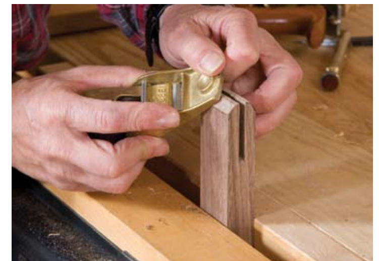
I bevel the top of the handle where it meets the tongue by planing across the board with a block plane to layout lines.
