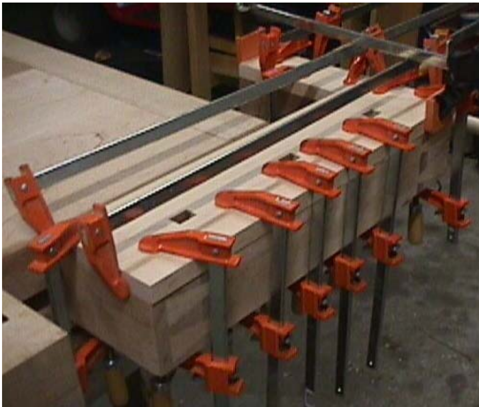
Clamping and gluing the top caps into place
