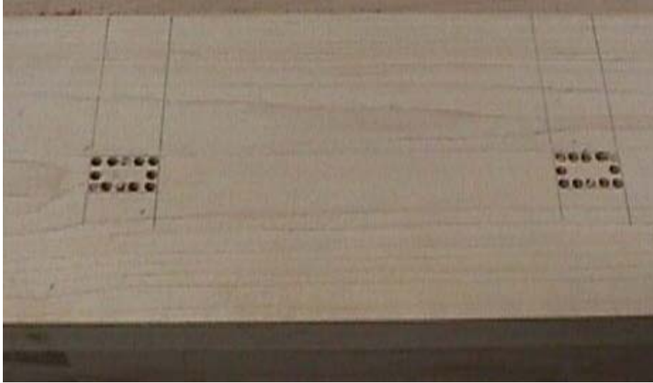
The holes drilled to help remove the waste
