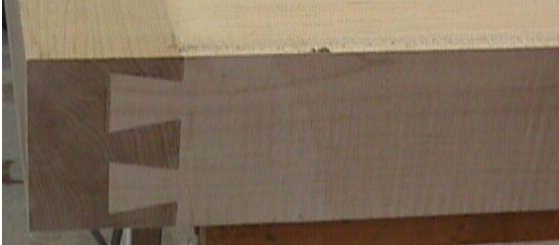
The dovetails on the back apron and back of the end caps.
