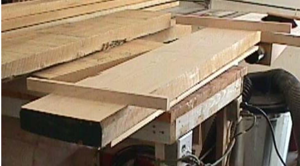
The Winding Sticks on the flat top of my board after planing. Notice the "flat" board which is nailed onto the bottom with wedges to keep it from rocking.
